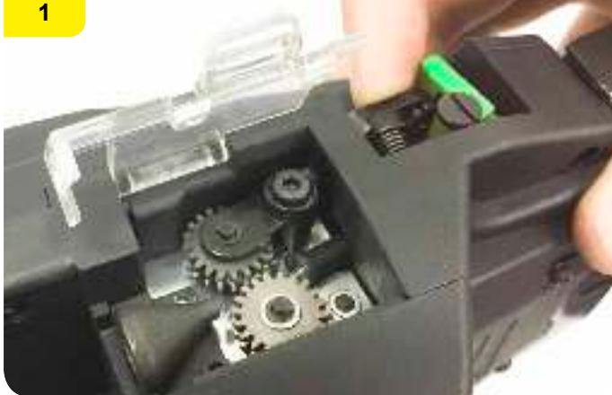
Unlock the reel stopper to open the reel stay door and load the wire coil.
