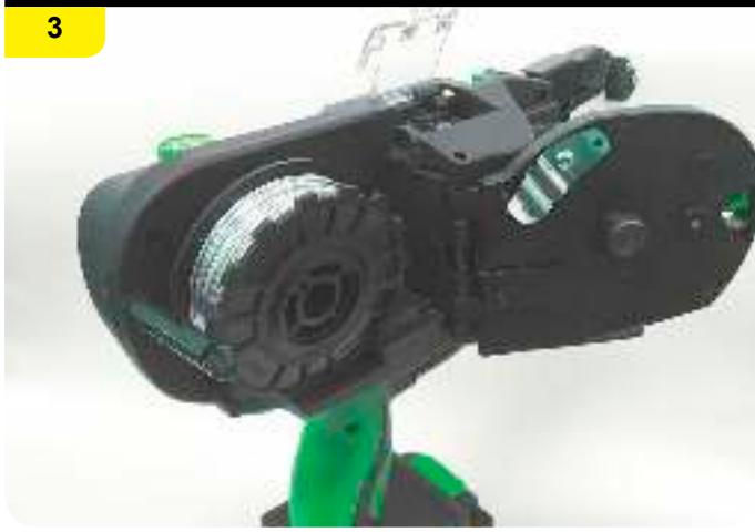
Insert the tip of the wire into the wire guide, through the gap of the feeding gears till the pipe and all the way into the machine upper jaw arm A (max. 70mm).
