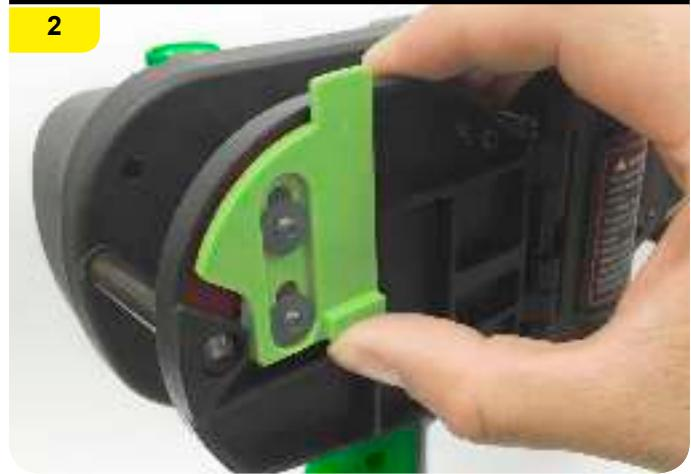
Once wire coil is loaded lock the reel stay door back again.
