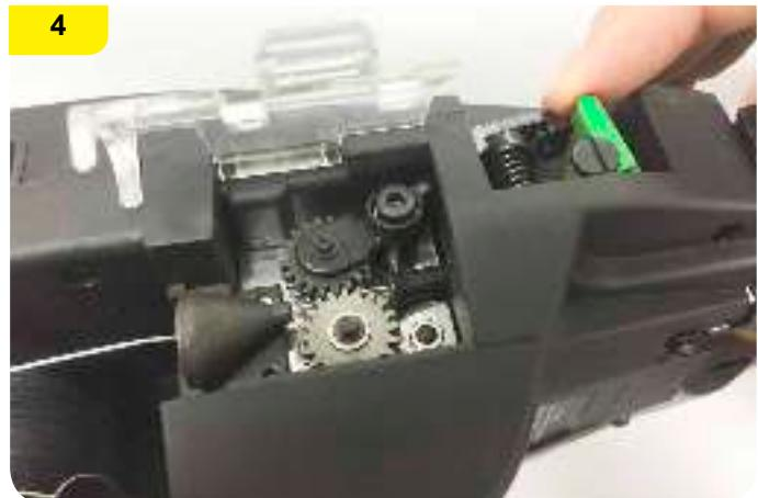
Push the release stopper to unlock the release lever, make sure the release lever is back to original position and the feeding gears are clamping the wire.
