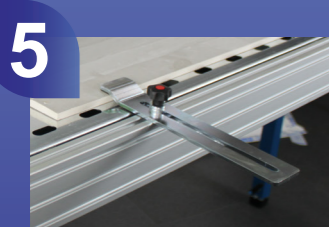
5 4 clamps set to hold the tiles while cutting
