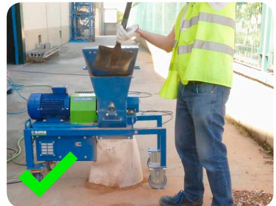
Do not disconnect the machine till it has already finished crushing, unless there is an emergency. If you disconnect the machine with traces of rubble inside the crushing chamber, the motor will not have enough power to get back on track.
