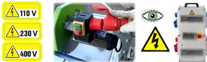
Once you have realised the previous steps and before placing the disk and manipulate the motor, it is necessary to check and adjust the rotation of the motor axis correctly, you have to plug the machine to the electricity and start it up, watching the rotation direction that must be clockwise.
