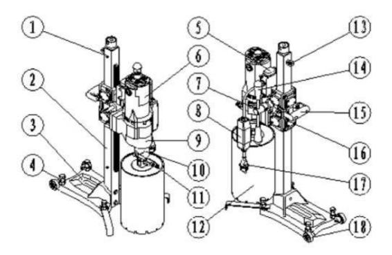
1.stop knob 2.column 3.base 4.leveling bolt 5.swich 6.motor
