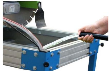
During cutting operations accumulate lots of dirt on the tray so the water should be changed as often as necessary to ensure the smooth operation of the pump and the perfect cooling of the blade, the tray features a drain plug that facilitates this operation.
