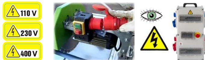
Once you have realised the previous steps and before placing the blade and manipulate the motor, it is necessary to check and adjust the rotation of the motor axis correctly, you have to plug the machine to the electricity and start it up, watching the rotation direction that must be clockwise.
