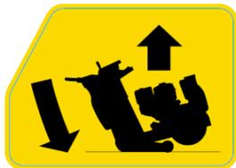
MONTÉE DE LA MACHINE LORSQUE LE VOLANT TOURNE DANS LE SENS ANTI-HORAIRE.
