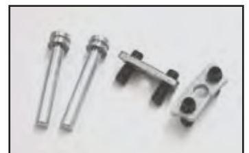
Angle selection pins with memory holders for 2 different angles programme.
