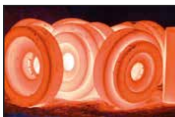
Inner components tempered for extended working life.
