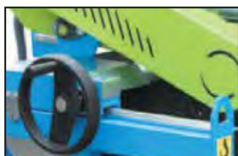
Handwheel operated mechanical feed.
