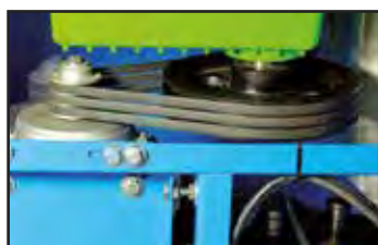
New easy and quick belts tightening system.
