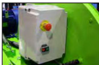
New star-delta motor starter.
