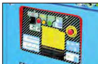
Protection shield for control panel.
