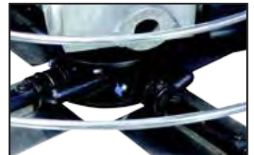
Blade holders include a lubricator nipple for an easier maintenance.
