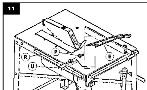
The graduation of the angle with which it wants to cut will be achieved by loosening the set screw of the support piece **P**, Fig.11 and turning it to the desired position.
