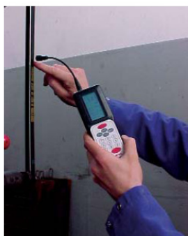
TENSION CONTROL BY VIBRATION METHOD
