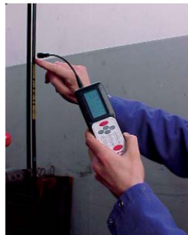
TENSION CONTROL BY VIBRATION METHOD
