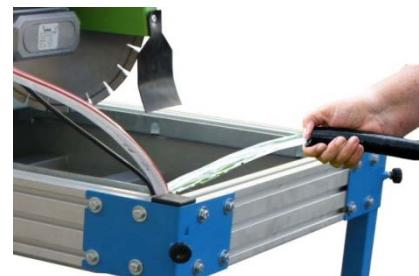
During cutting operations accumulate lots of dirt on the tray so the water should be changed as often as necessary to ensure the smooth operation of the pump and the perfect cooling of the blade, the tray features a drain plug that facilitates this operation.
