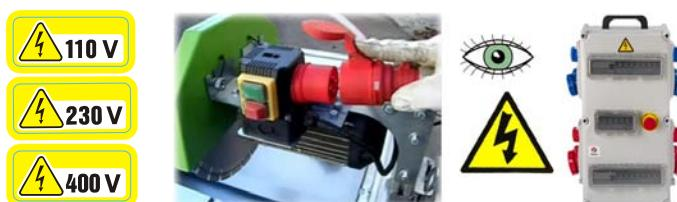
Once you have realised the previous steps and before placing the blade and manipulate the motor, it is necessary to check and adjust the rotation of the motor axis correctly, you have to plug the machine to the electricity and start it up, watching the rotation direction that must be clockwise.
